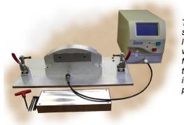
TME Solution single-port leak tester with custom fixture for testing heavy industrial products.
